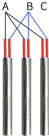
220V connected to 220V in parallel
